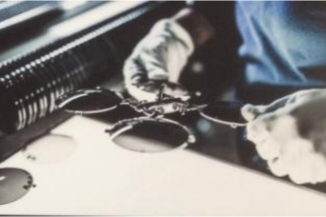
Moulded lenses are checked and separated
