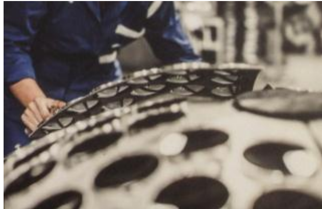
Lenses are placed on the support of the oven
