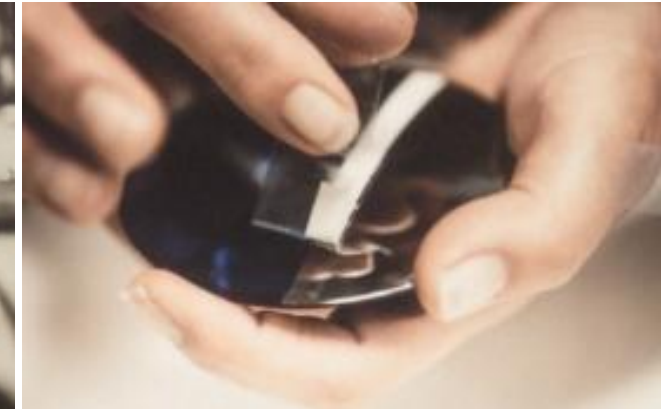
The stamping is hand-removed and lens quality is controlled. The lens is then cut at the right dimensions and mounted on the frame
